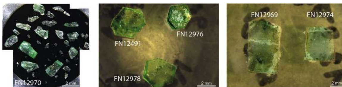
Figure 12: Sample preparation. (Left to right) Crushed samples for SEM analyses; the bigger pieces were verticalized during preparation and silver pasta applied on the side to avoid electron accumulation (air, brightfield). The three samples sliced ( \perp C ) and casted in epoxy resin for microprobe analyses; note the bubbles and brown polishing diamond powder occurring around the slices despite the care taken (air, brightfield). The two halved ( \parallel C ) samples for microprobe analysis with a large fracture through FN12969 (air, brightfield).
